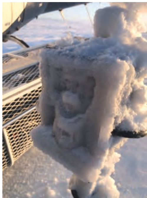
Example of frozen trail cameras, necessitating the need for mid winter maintenance.
