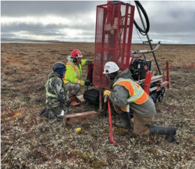
Field Crew Using A Shock Auger Drill, Rankin Inlet, NU.
