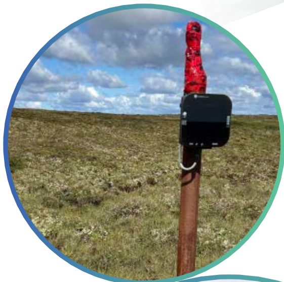
Thermistor before conduit protection added.
